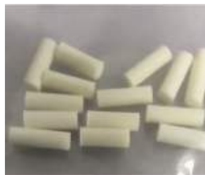
Figure 1. ChemoSeed – 6mm in length, 2mm in diameter
